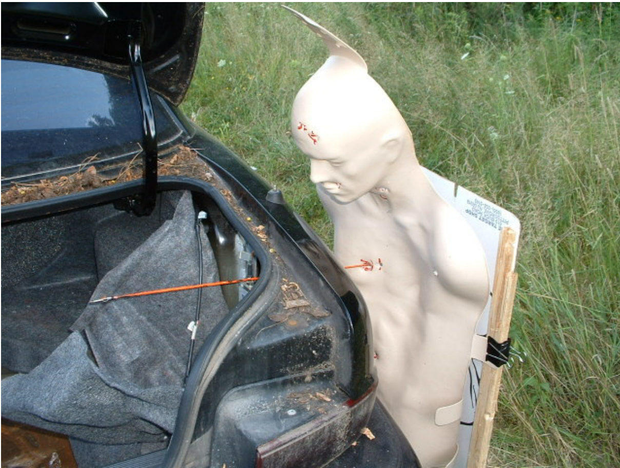
Pistol ammunition penetrated both sides of the trunk and the target.
