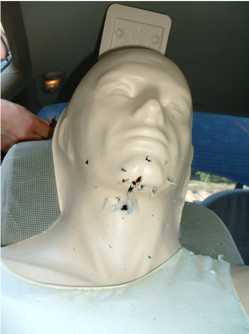
.223 Full Metal Jacket fired through windshield produced numerous metal and glass fragments.
