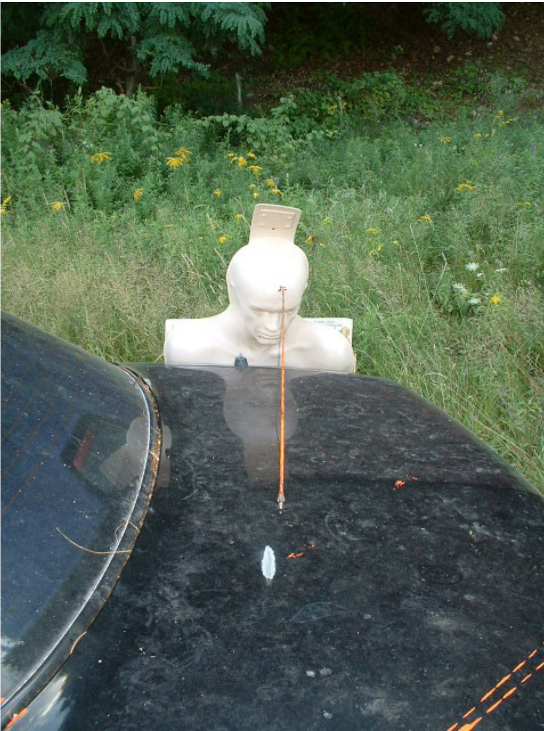
Pistol ammunition deflected off of the trunk striking the target in the head.
