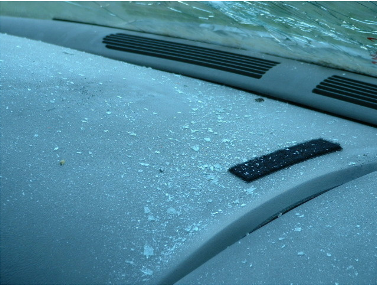
Glass fragments produced when the windshield was struck by several bullets...
