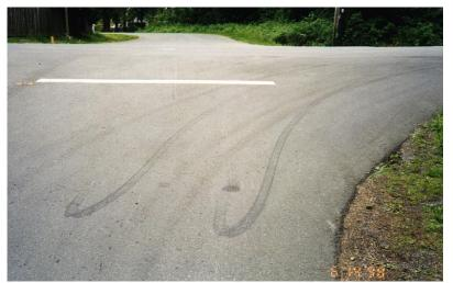
Unlike a skid mark, a driver can steer the vehicle as it leaves an acceleration scuff. Sometimes the beginning of the scuff mark will resemble a hook (left). This occurs when the vehicle is going backwards when the power is applied to the wheels. spin Although the wheels
