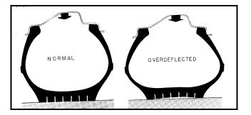
**Overdeflection** causes more friction at the edge of the tires, making the outside edges of the skid mark darker (below). Since the rear tires are being "lifted", they become **Underdeflected**. Because there is less weight on the rear tires, there is less friction. This causes a rear tire mark to be lighter and not as wide as the
