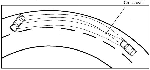
A yaw mark will be noticeably different from a skid mark. Obviously it will be curved. A yaw mark will also have diagonal striations and a scalloped edge (right). These marks are generally shorter than skid marks.
