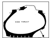
This distinct mark is caused by the outward weight shift of the car causing the side-rib and side-wall of the tire to cuff against the road surface (right). Because the tire is continuously rotating, bringing a new area of tire in contact with the road surface, there is less friction and the mark will generally be lighter than a skid mark with the darkest marks are from normally from tires on the
