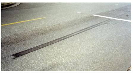
scuff on hard pavement will leave a distinct mark. The beginning of the mark will be dark and then get lighter as traction is gained and there is less friction (above, right).
