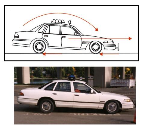
These parallel but opposite forces pitch the vehicle forward, causing weight from the rear wheels to shift to the front wheels (above). Because of this weight shift, the front suspension compresses, causing the front end to dip. As you can see, the rear suspension expands, causing a lifting of the rear tires. On average, about 60% of the weight is now on the front tires. This leaves 40% on the rear tires. Because of this weight shift, front and rear tires leave distinctly different skid marks.
